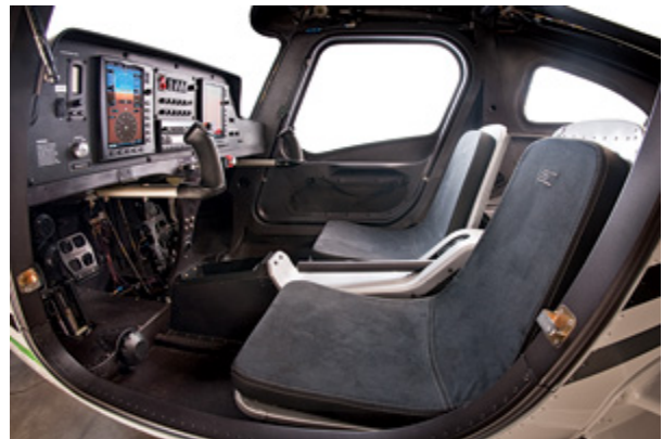
The 162's seats are fixed; however, both sets of rudder pedals are adjustable.
