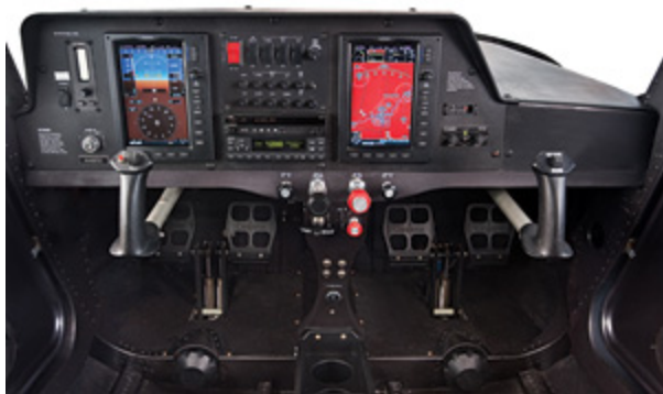
The Skycatcher's panel is built around the G300, a scaled-down version of the G1000.
